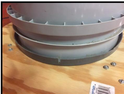
The picture below illustrates how the lid of the bucket is bolted to the plywood.
